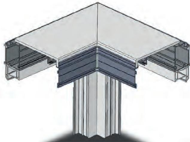
Offer up the Underclad and clip the Ring Beam Internal Trim into place.
